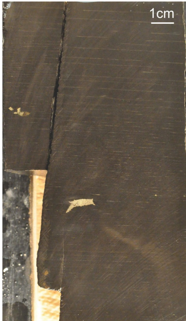
Figure N-09-1. Siliceous shale with pyrite streaks and upright calcite-lined fracture, 1670.2 m MD
