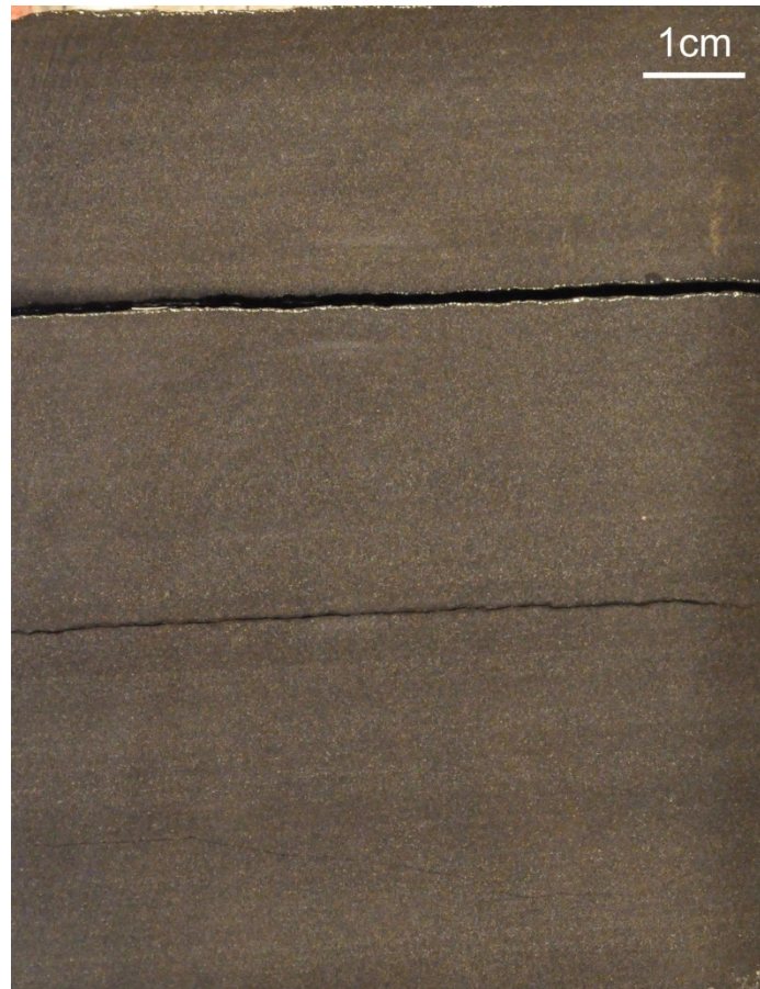
Figure N-09-9. Laminated calcareous hard siltstone, 1749.45 m MD
