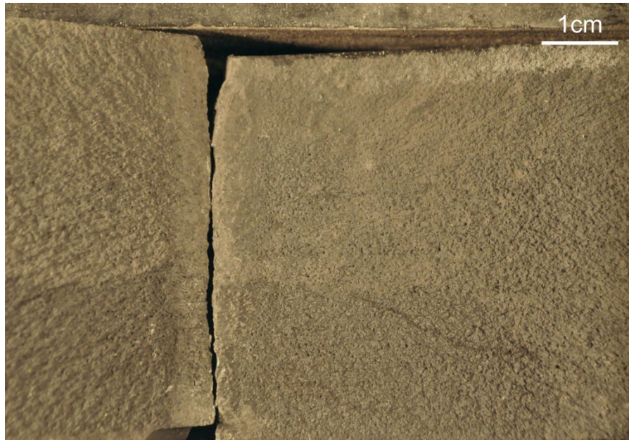
Figure N-09-14. Upright fracture plane in hard shale (mudrock), 1766.8 m MD
