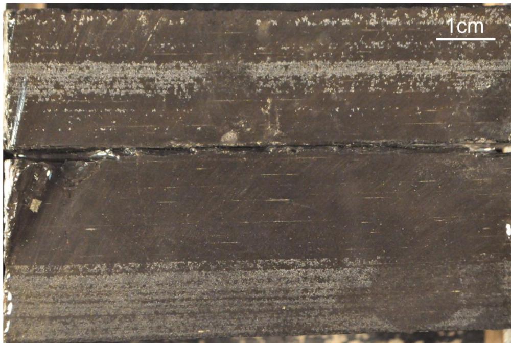
Figure N-09-5. Calcareous shale with lamination emphasized by diagenetic calcite aggregates (“stellate calcite”), 1714.4 m MD
